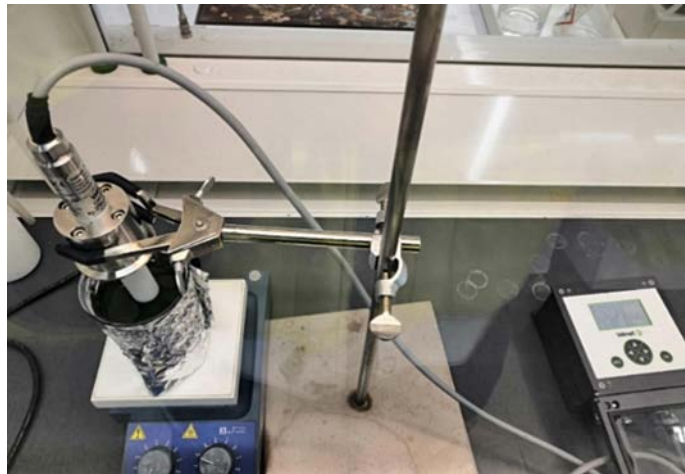
Figure 11. Studying conductivity behavior in different temperatures.
