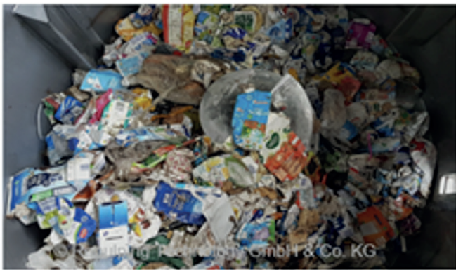
Figure 12. Input (left) and output (right) of a repulper after separation of liquid board packaging with a cavitation pulper (Mod. Repulping Technology GmbH 2021)
