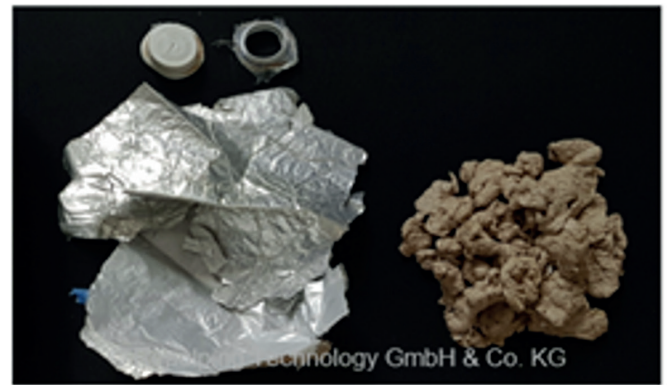
Figure 12. Input (left) and output (right) of a repulper after separation of liquid board packaging with a cavitation pulper (Mod. Repulping Technology GmbH 2021)
