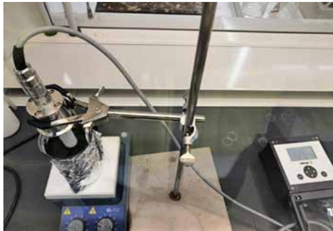
Figure 11. Studying conductivity behavior in different temperatures.
